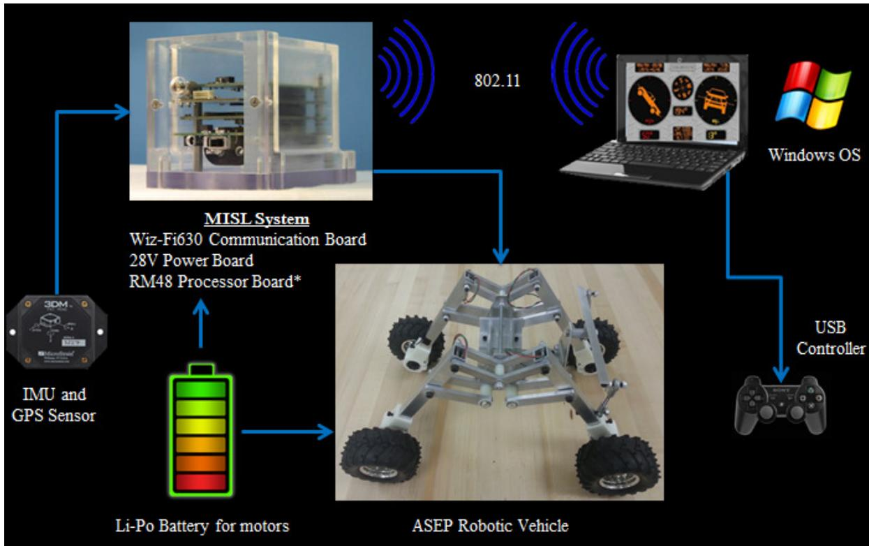
Figure 5: Conceptual Block Diagram
