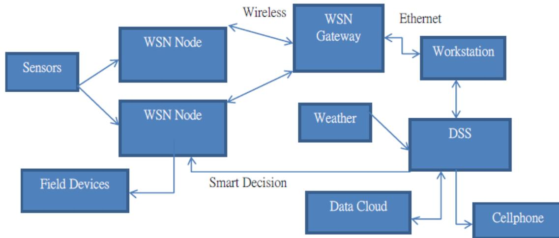
Fig. 2 ICT of the smart irrigation DSS
