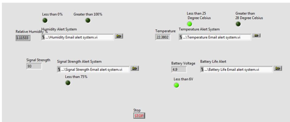
Fig. 5 LabVIEW Front Panel
