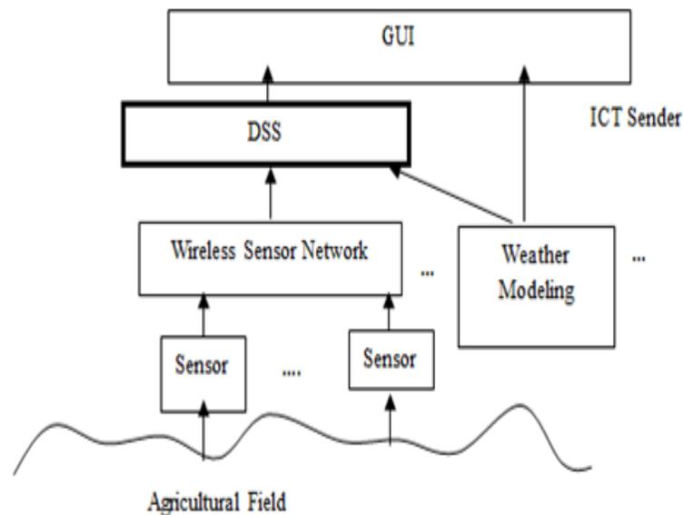
Fig. 1 Smart irrigation DSS schematic diagram
